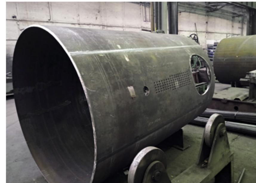
**The coned section with the steam collector (banjo dome).**
