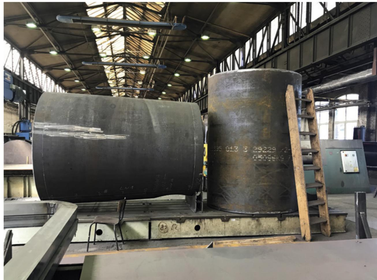
**Taper and parallel boiler barrel sections.**
