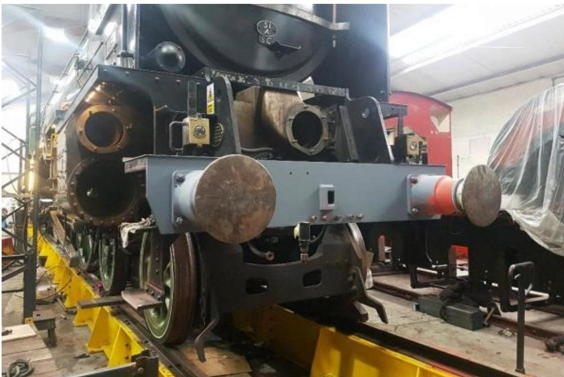
Following the cylinder re-bore, the front buffer beam was re-installed - Graeme Bunker-James
