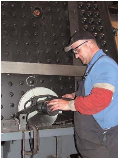
the correct clearance. The only areas where the boiler is significantly different to the original type is the front lower sides of the firebox which has resulted in the need to shave a small amount off the inside edges of the reverse curved section of the running plate to clear the cladding.
