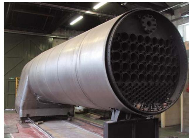
*Boiler cladding sheets trial-fitted to the boiler © David Elliott*
