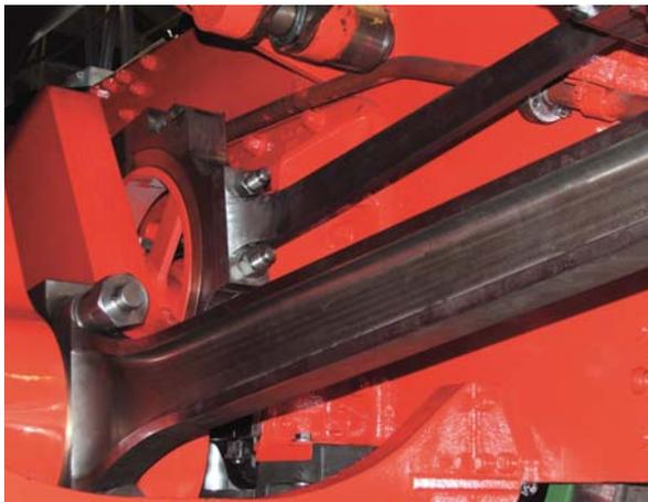
*Trial fit of the inside connecting rod and eccentric*
