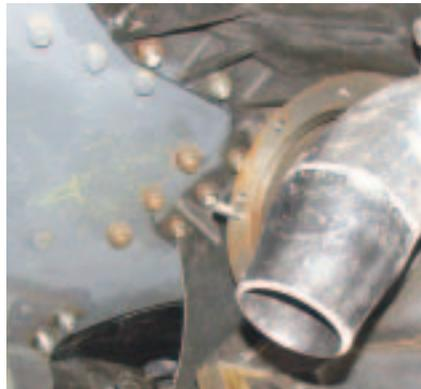
Exhaust injector steam pipe
