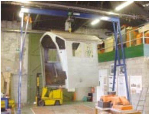
The cab is suspended from the new electric hoist prior to refitting to the locomotive
