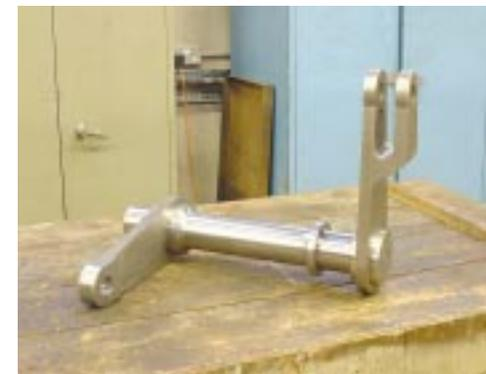
The reversing bell crank trial assembly on the bench
