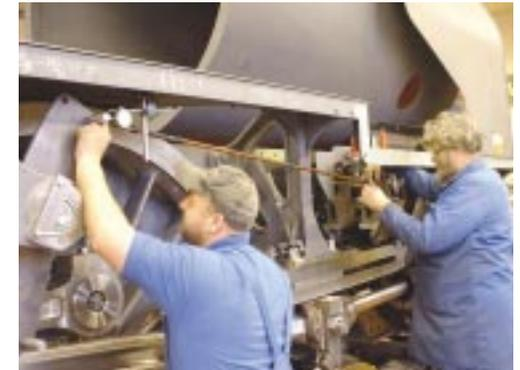
Mick and Ian use the inside micrometer to measure between the pins on the radius rod and the reference point
