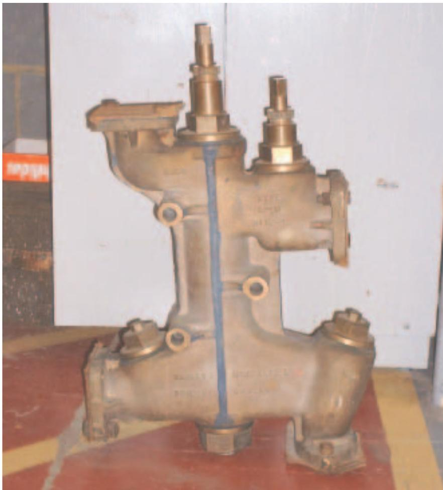
*Above: Sculpture in bronze:* A brand-new Davies & Metcalfe LM-type 12mm injector, one of two the trust has bought. As mentioned in *TL9*, these Lifting Monitor injectors are preset and then need no further adjustment when they are turned on. They were proved in everyday service on Bulleid Pacifics and Thompson B1s. *(photo: David Elliott).*
