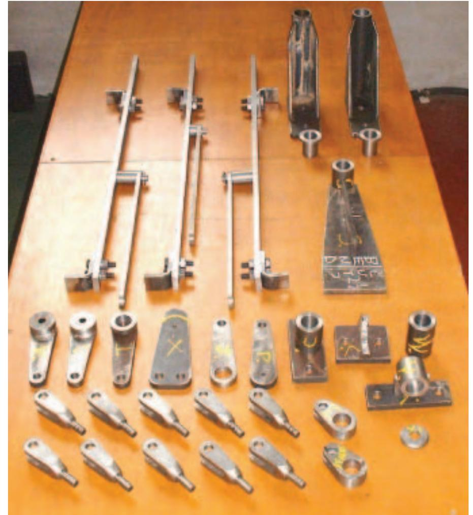
**Above: Really know your draincocks!** The picture shows how busy the Draincock Gang has been, led by Mike Wood, our Works Manager. This pull-rod assembly opens the valves that release condensate from the cylinders before starting.
