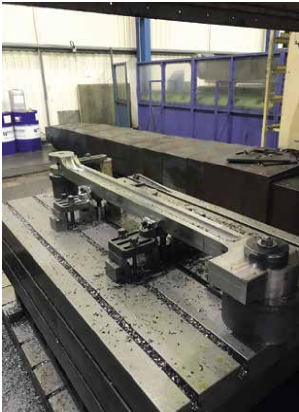
The leading coupling rod at an advanced stage of machining.
