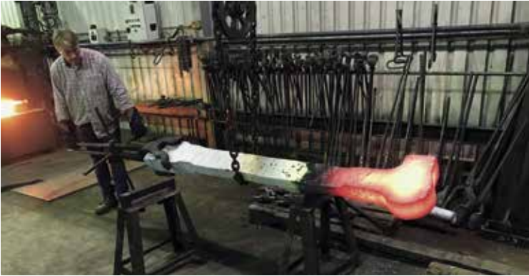
Forging coupling rod blanks at Stephensons.
