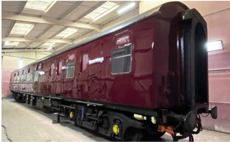
Above: The support coach is rubbed down in the Carnforth paintshop.
