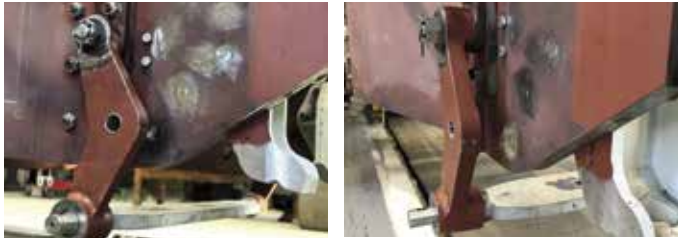
The two trailing brake hangers and brake stay fitted to the frames.
