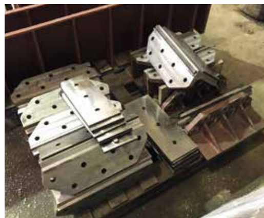
Tender hornguides with manganese steel lines welded in place.
