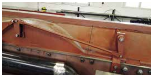
Trial fitting of front and rear engine brake cross shafts.
