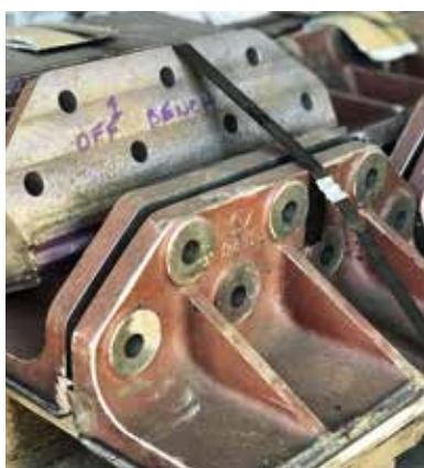
Tender hornguides with manganese steel lines welded in place.
