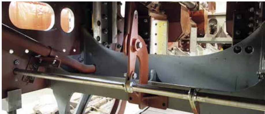
Cylinder drain cock actuating linkages.
