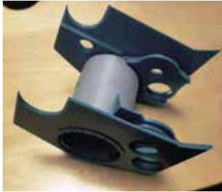
The partly assembled scale model of the cylinder block.
