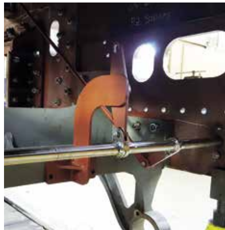
Cylinder drain cock actuating linkages.
