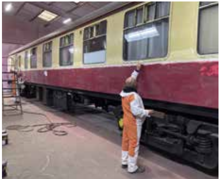
Above: The support coach is rubbed down in the Carnforth paintshop.
