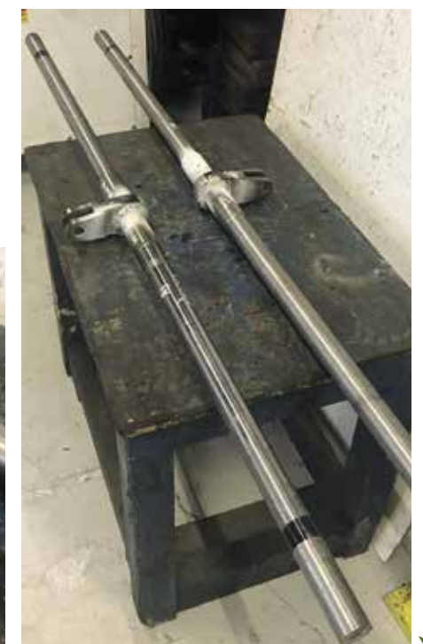
Right: Regulator cross shafts with the cranks welded on.
