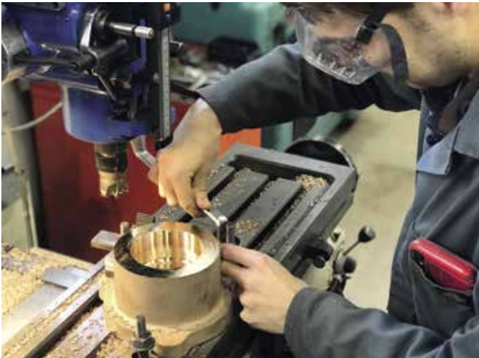
Above: Ed Laxton machining a brake cross shaft bronze bush.
