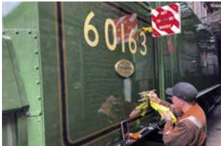
Ian Greenan applies the RA number to the cabside.
