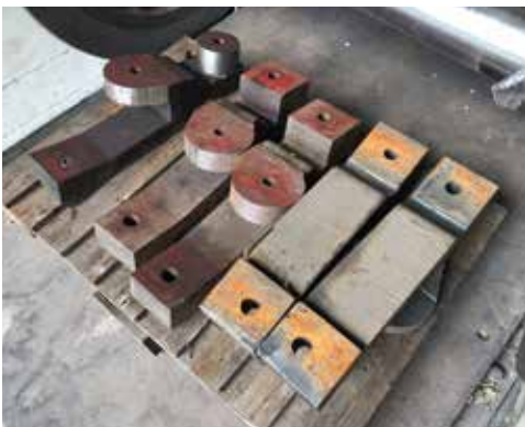
Right: Part-machined brake hanger profiles.
