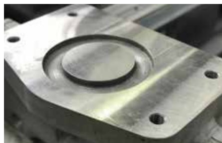
Above: The pony truck crosshead and the machined surface of the pony truck.
