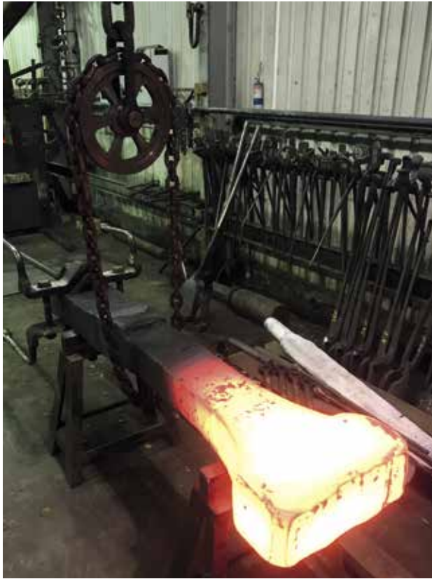
Above: The middle connecting rod is forged.
