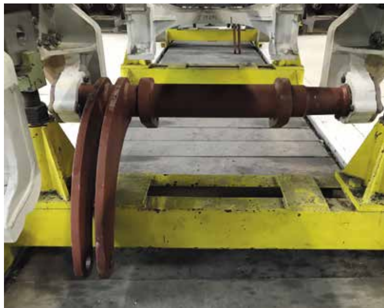
Trial fitting of front and rear engine brake cross shafts.
