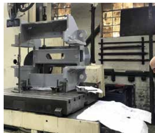
Machining the pony truck on the horizontal borer at NVES.
