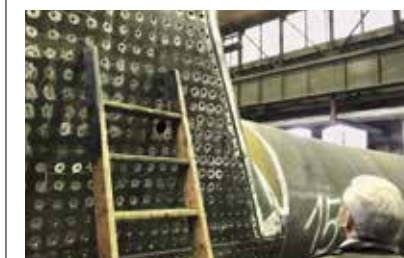
Above: First boiler being assembled at DBM.
