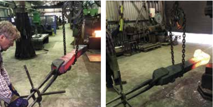
Forging coupling rod blanks at Stephensons.
