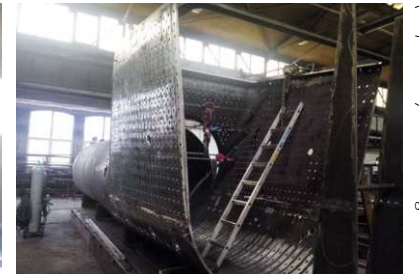
The firebox is then offered up to the boiler barrel...
