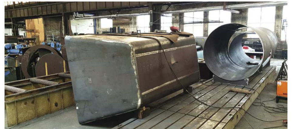
The inner firebox welded up.
