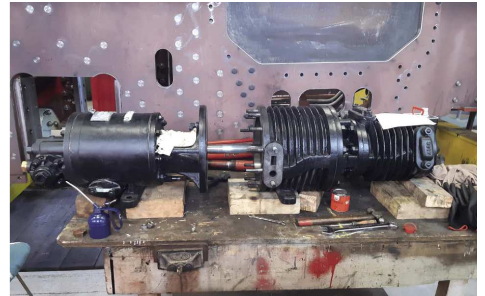
Air pump split with new stud fitted.
