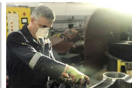
Ian polishing the leading coupling rods.
