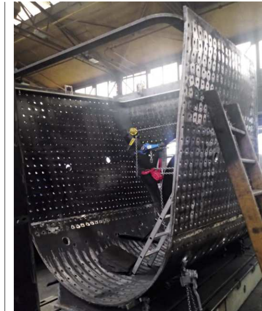
The firebox is then offered up to the boiler barrel...
