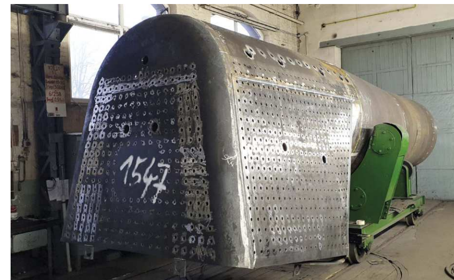
Above: The boiler shell in Meiningen's X-ray room for weld checking.
