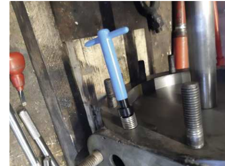
Helicoil and insertion tool.
