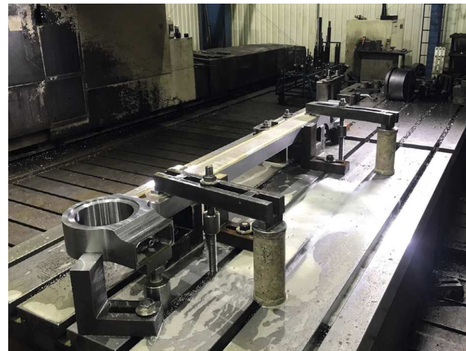
Above: The leading connecting rod being machined at Stephenson's.
