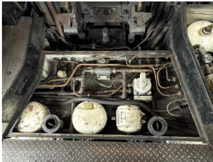
The cab floor lifted to reveal the air receivers.
