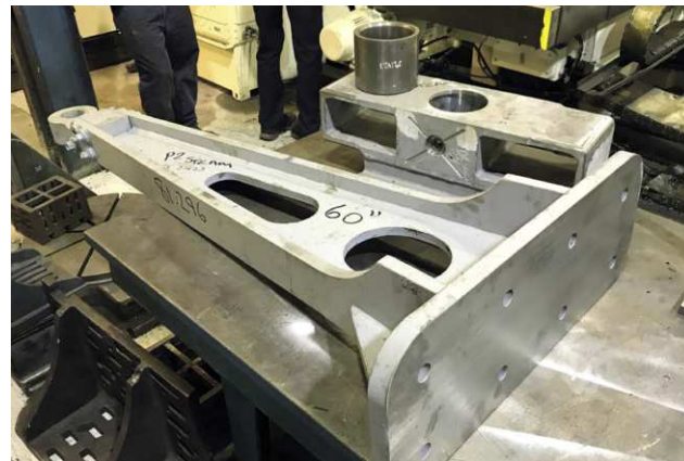
Progress machining the pony truck steering arm at North View Engineering.
