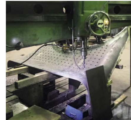
Above: Boiler #2 (or is it #3?). Drilling the outer firebox throatplate for stays.
