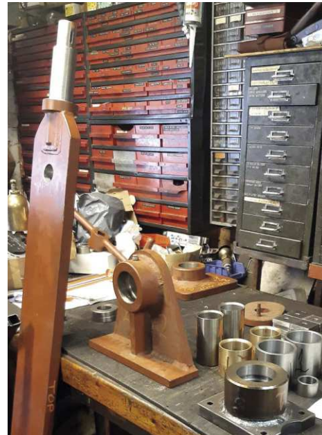
Above: Tender brake stay and bearing details.
