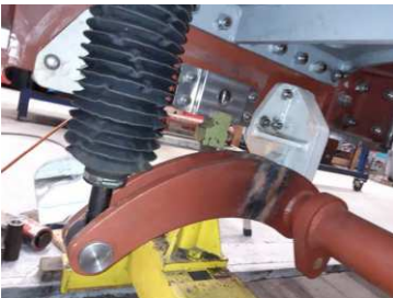
Brake cylinder and cross shaft with piston rod fully extended.
