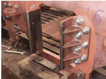
Above: Tender brake stay and bearing details.
