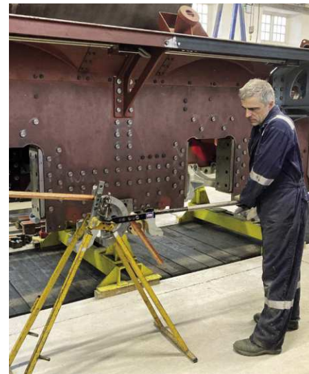
Ian Matthews bending copper pipe for the air brake system.
