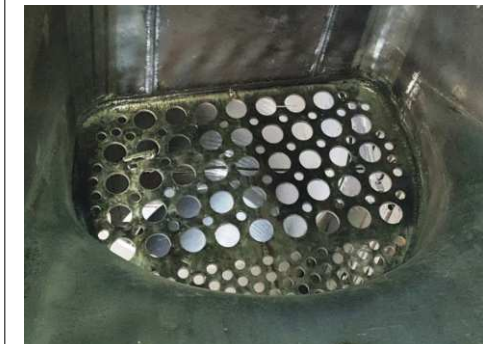
Above: Welded seams detail, firebox.
