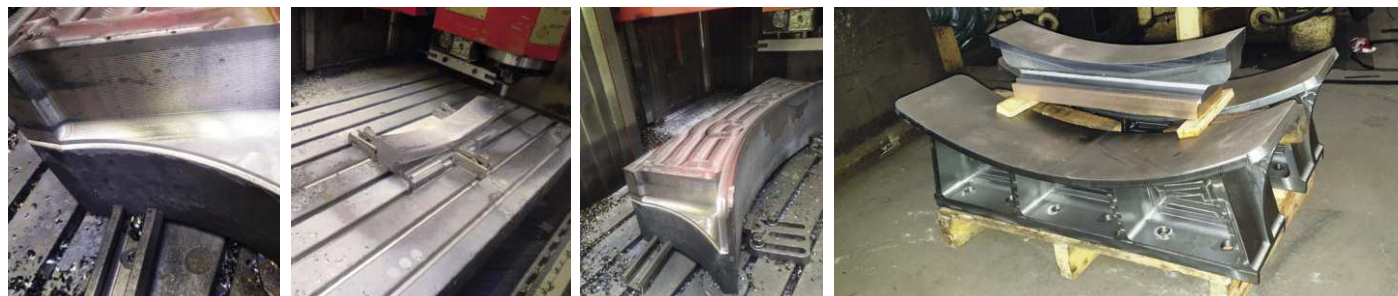
A series of photos showing the machining of the boiler supports from solid steel.
