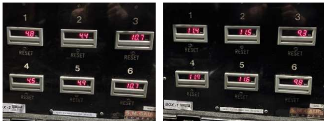
These pictures show the final weights, starting on the left with the front of the engine and working across to the rear on the right, the top row shows the RHS of the engine and the bottom row is the LHS.
