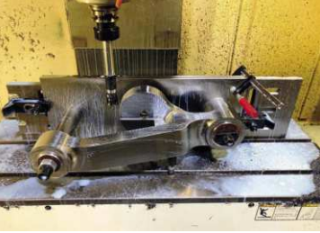
The 'Y' shaped brake hanger being machined.
