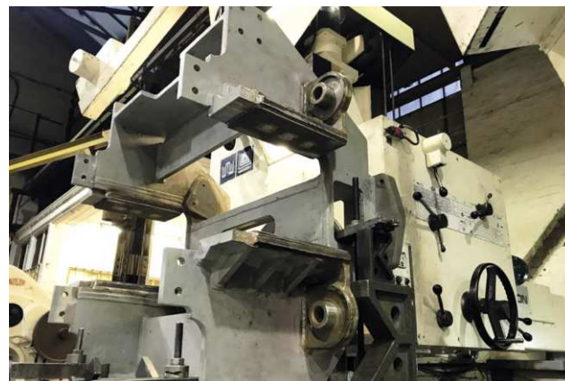
Machining the pony truck hornguides at NVES.
