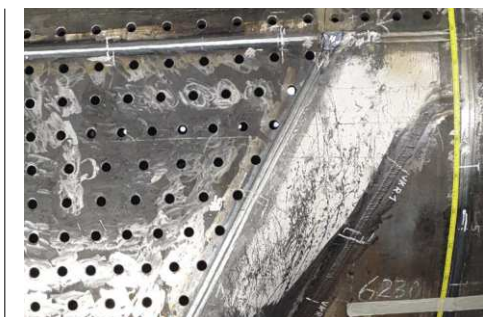
Above: Welded seams detail, firebox.
