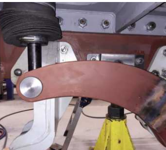
Brake cylinder connected to rear brake cross shaft.
