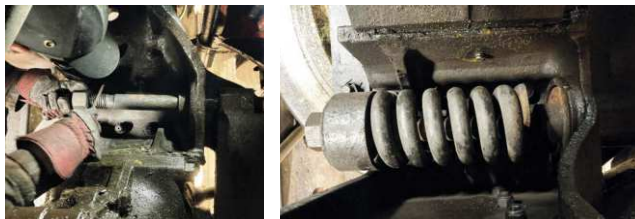
The pictures show Ian dressing one of the bolts (left) and reassembled with spring (right).
