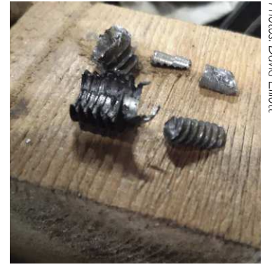
Pieces of broken stud and stud extractor.
