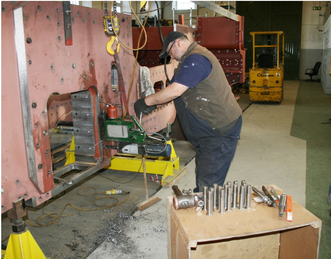
The hornblocks being fitted to No. 2007's frames
