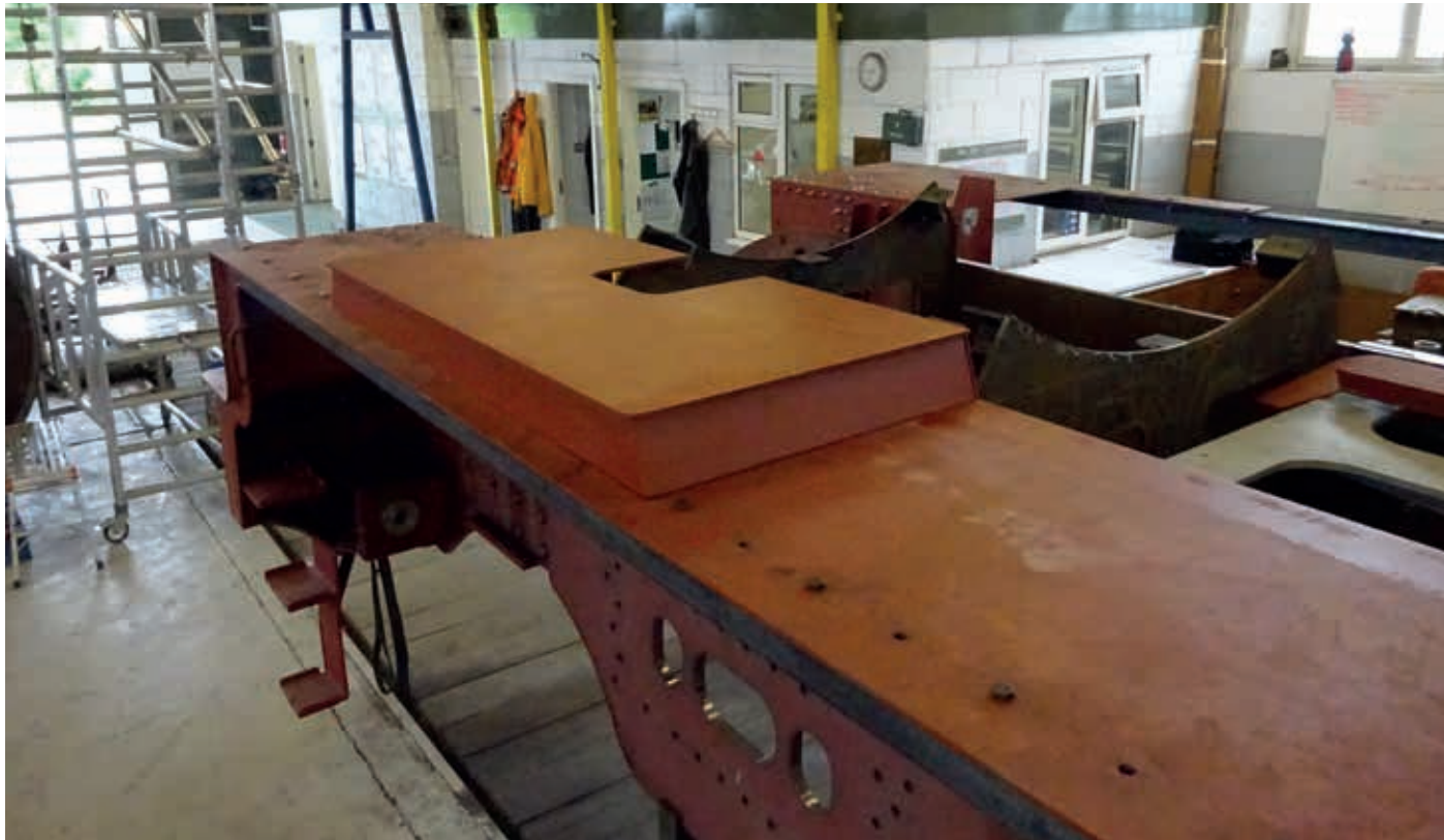
Above: The raised platform over cylinders.
