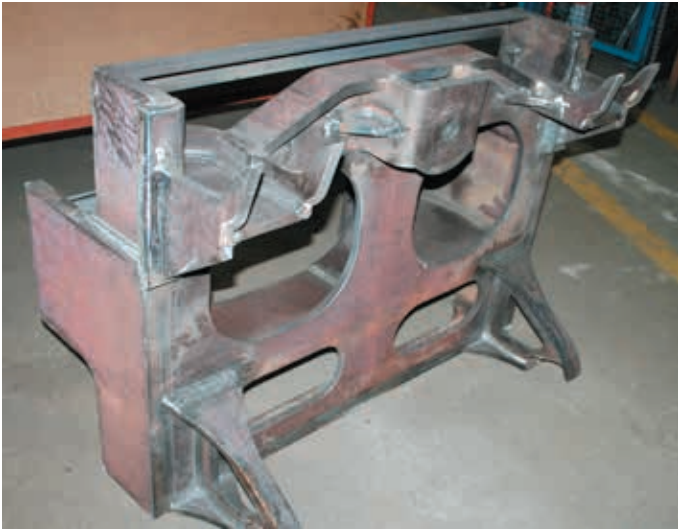
Above: Leading brake stay nearing completion of fabrication.
