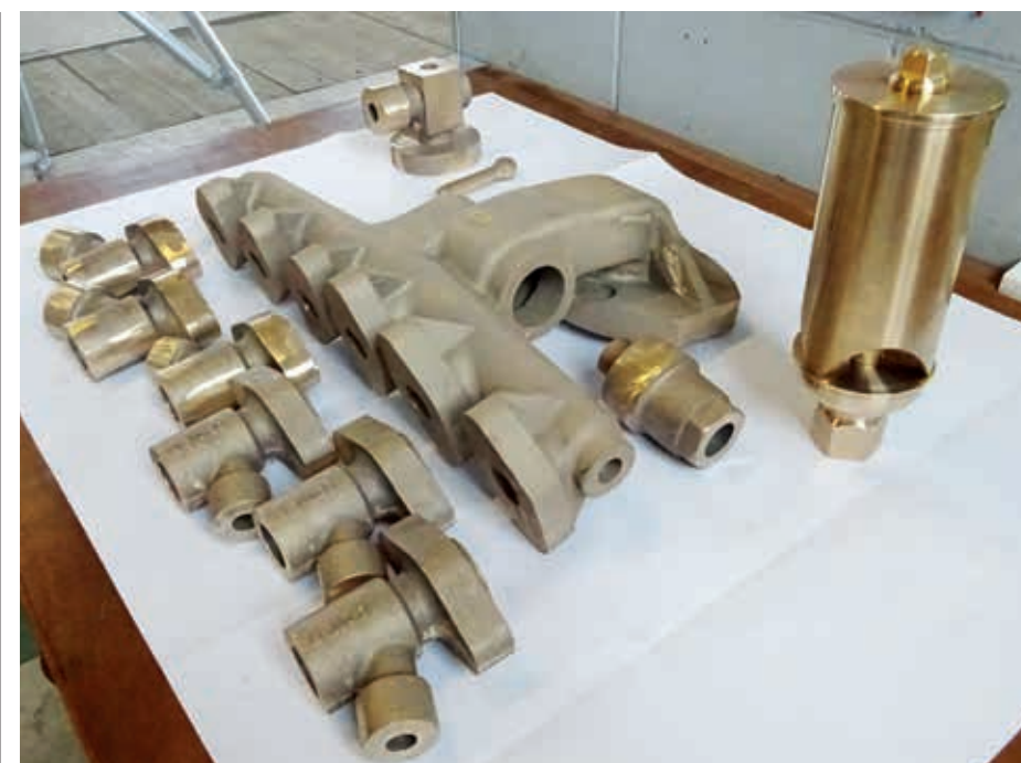
Above: Castings for the steam stand and fittings and the chime whistle.
