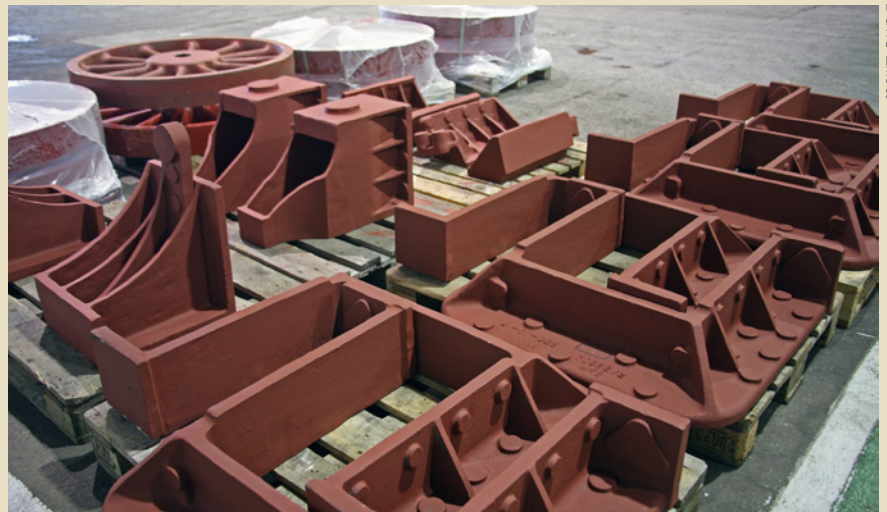
Some of the many castings for frame stays, horn guides and wheels at William Cook Cast Products.
