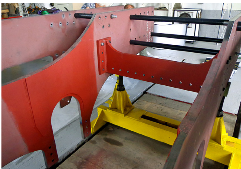
One of the fabricated frame stays in place between the frames.
