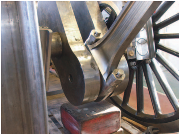
The Trial Fit of the Inside Big End
