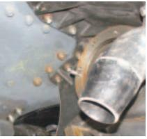
Exhaust injector steam pipe
