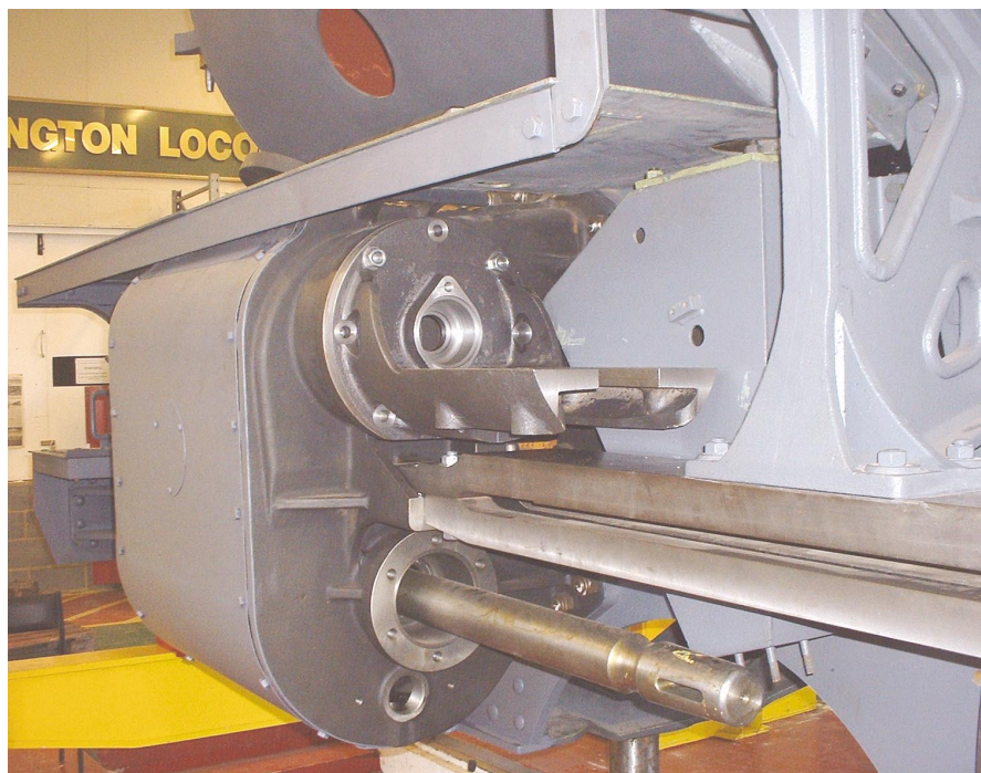
Above: Trial fit of the rear steamchest cover, April 2003 (photo: David Elliott)
