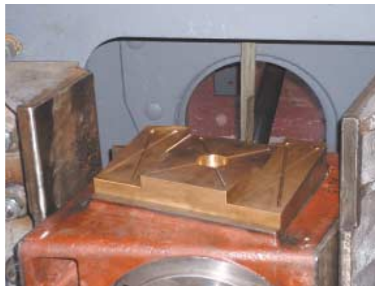
Left: The weird and wonderful Cartazzi wedge. Unlike a radial axle, its various profiles are all straight lines – much less trouble for the workshop. (photo: David Elliott)
