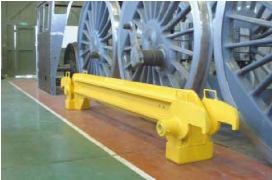
The new rear lifting beam as delivered to Darlington Works following its certification to 40 tons SWL, after shot-blasting and painting. (photo: David Elliott)
