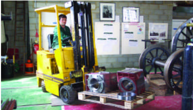
The Works fork-lift truck is seen lowering a pallet with the Cartazzi axleboxes, unloaded on their return from North View Engineering after machining. (photo: Barry Wilson)
