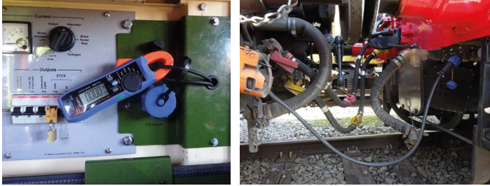
Above left: Bluetooth clamp ammeter trial fit, ready for recording ETCS current during Cambrian testing. Above right: Coach-to-locomotive jumper in place between the vehicles.
