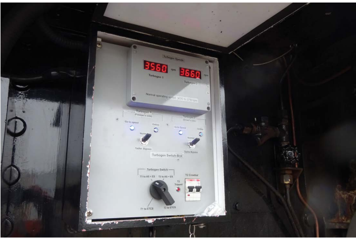
Turbogen speedometer displays showing old turbogen running at 3560rpm and new one at 3660rpm.
