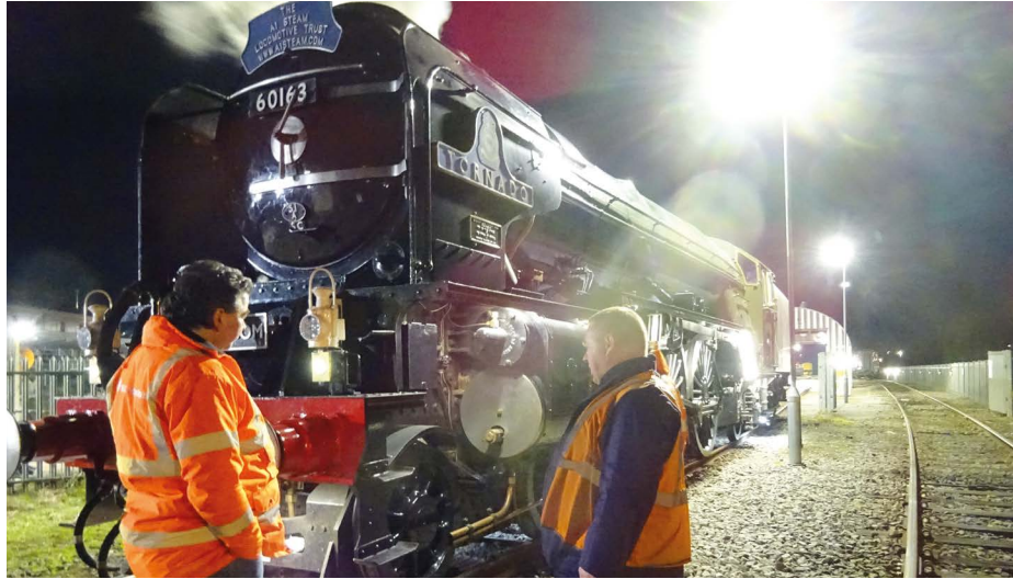
Above: Logging meters in place ready to record the ETCS voltage and current.
