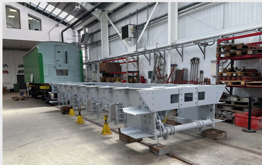
The P2's tender frames await the fitting of the balanced wheelsets.
