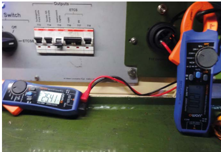
Above: Logging meters in place ready to record the ETCS voltage and current.
