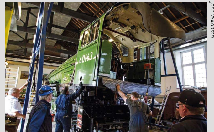
The cab is lowered onto the frames in Spring 2015.
