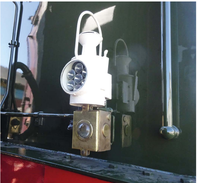
Headlamps fitted to the tender in preparation for tender-first working back from Newtown.
