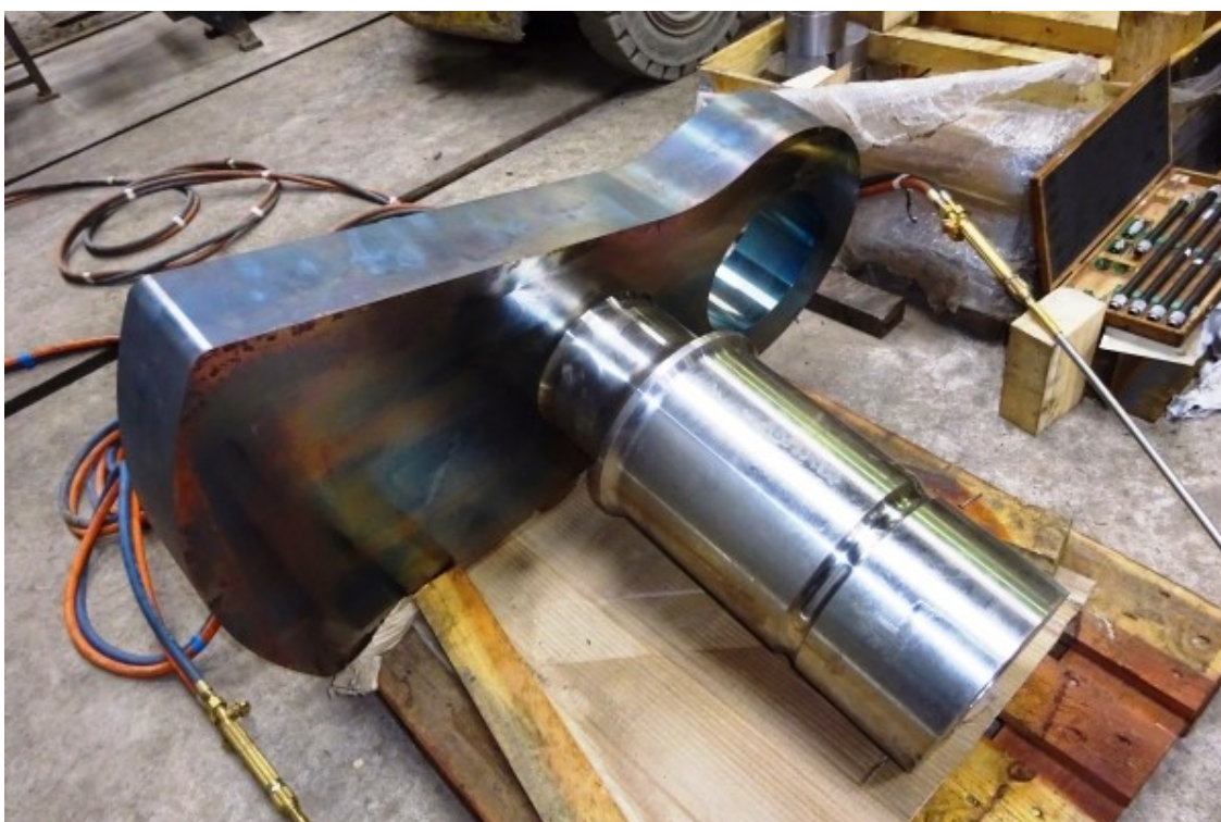
The partly assembled crank axle at SDE - David Elliott
