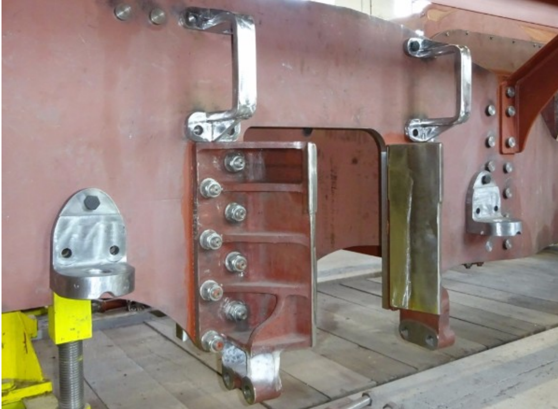
The spring hanger brackets in place on the frames - David Elliott
