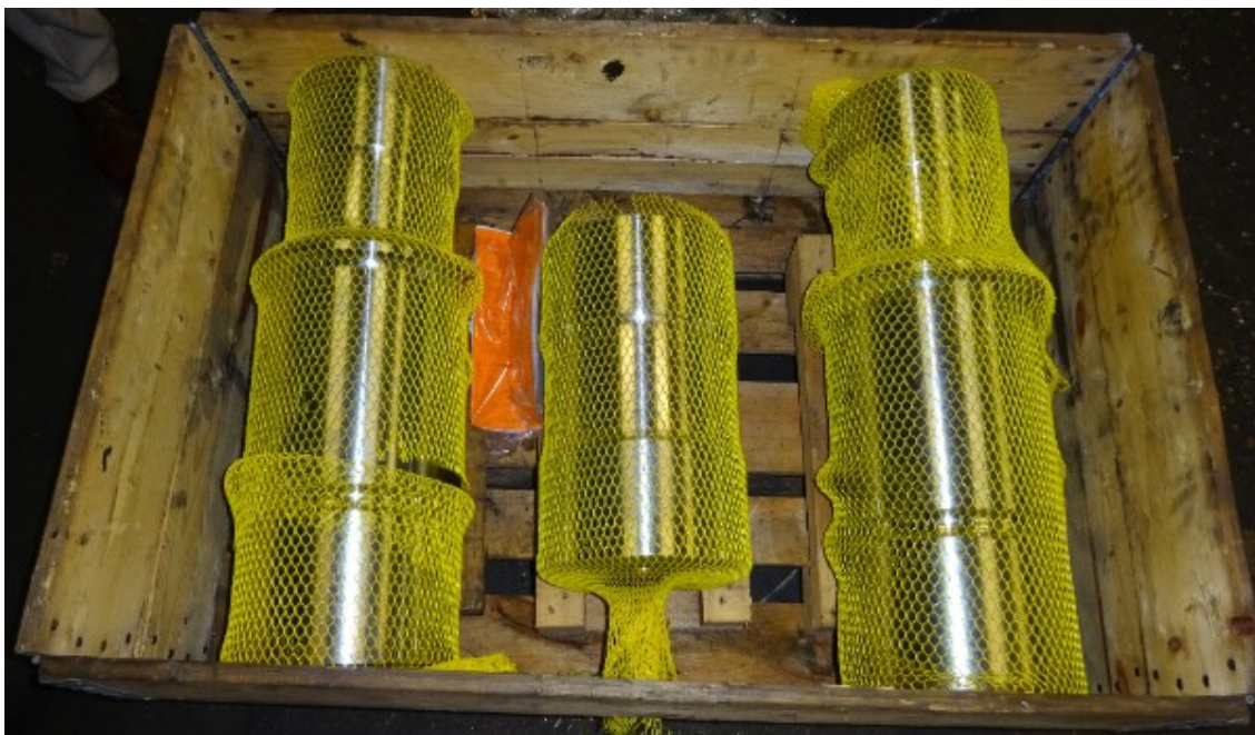
Crank axle components have been machined at Unilathe - David Elliott
