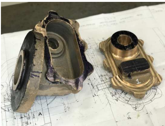
Welding progress on the outer firebox at DBM; proof machining of the stuffing boxes at DLW - DBM/A1SLT
