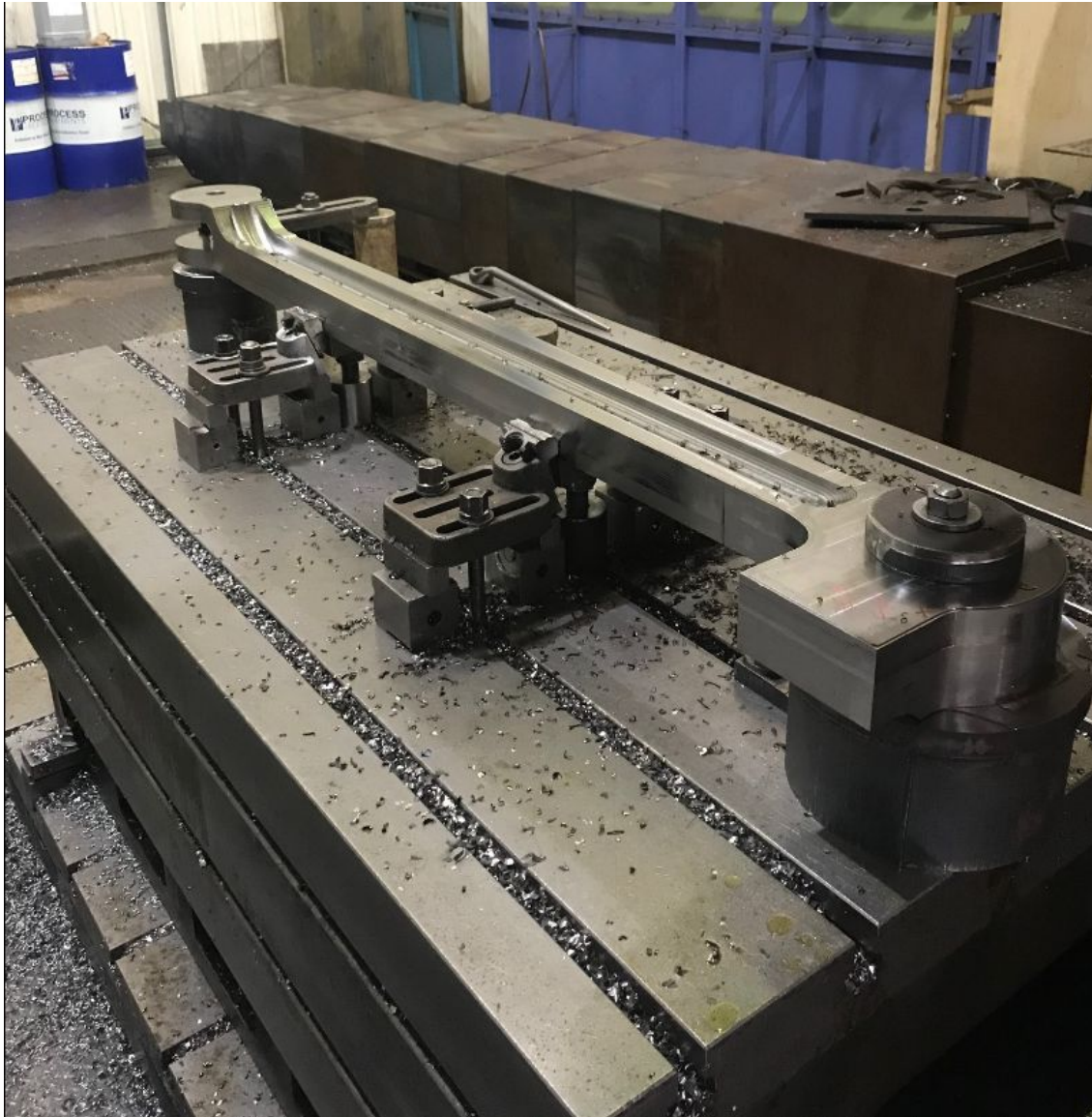
A leading coupling rod in the advanced stage of machining at Stephenson (Engineering) Ltd - Robert Stephenson/A1SLT
