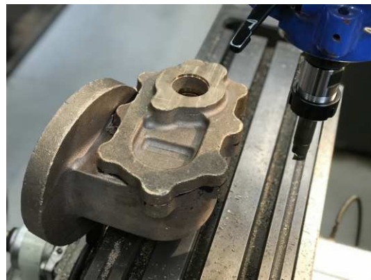
Welding progress on the outer firebox at DBM; proof machining of the stuffing boxes at DLW - DBM/A1SLT
