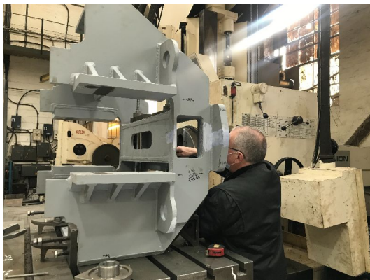
The pony truck frame on the horizontal borer at NVES - A1SLT
