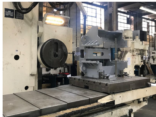
The pony truck frame on the horizontal borer at NVES - A1SLT
