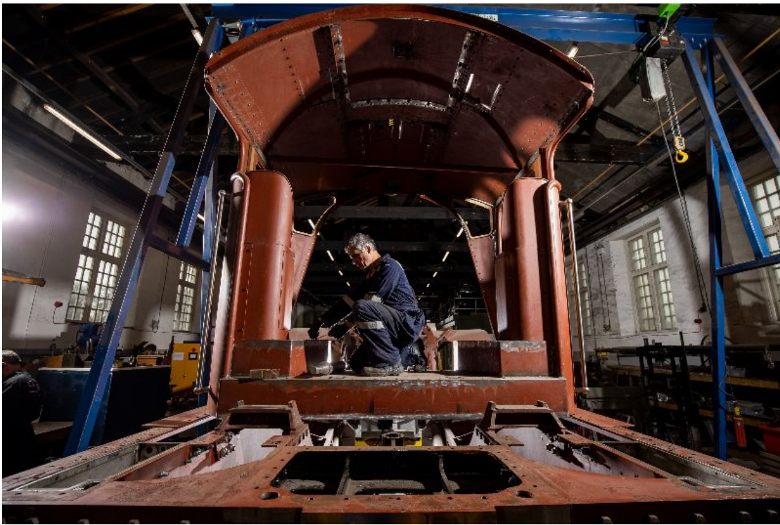
Ian Matthews checking bolts in the cab floor plate - CAG Photography/A1SLT
