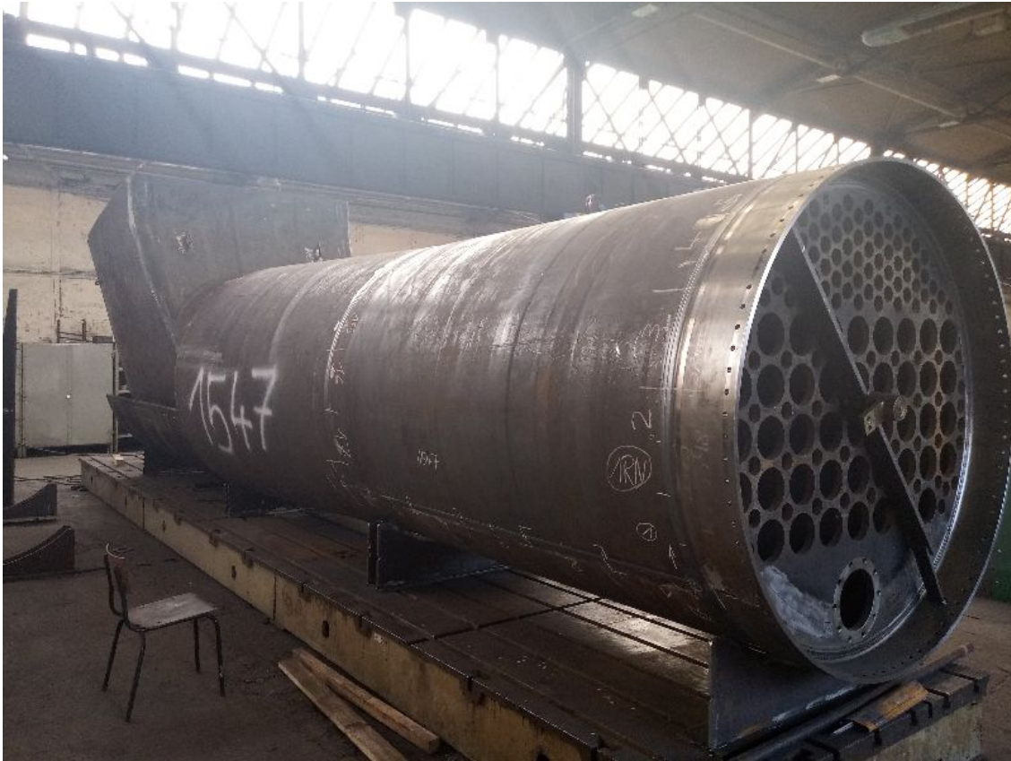
The first new boiler being assembled at DB Meiningen - DBM/A1SLT
