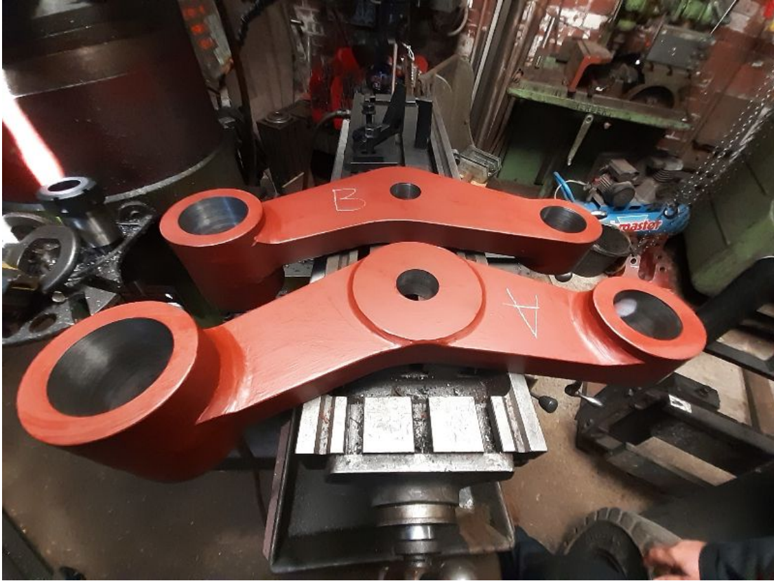
Engine rear brake hangers before fitting bushes - A1SLT
