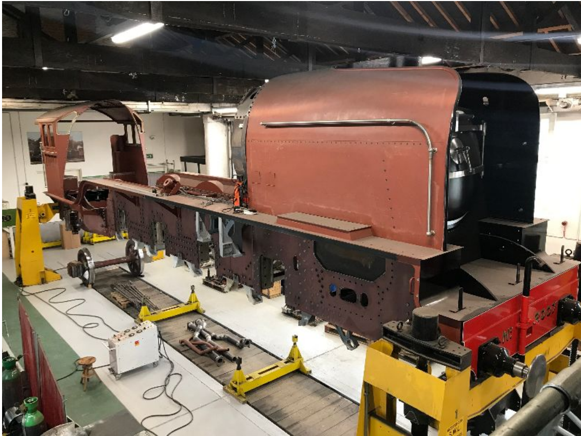
A 'Flying Mikado' (aka No. 2007 Prince of Wales ) awaiting her wheels being 'fitted beneath' - A1SLT
