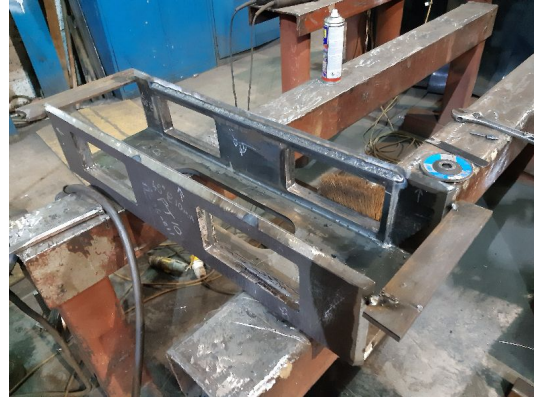
Cartazzi wheelset and spring plank assembly; pony truck frame fabrication - A1SLT
