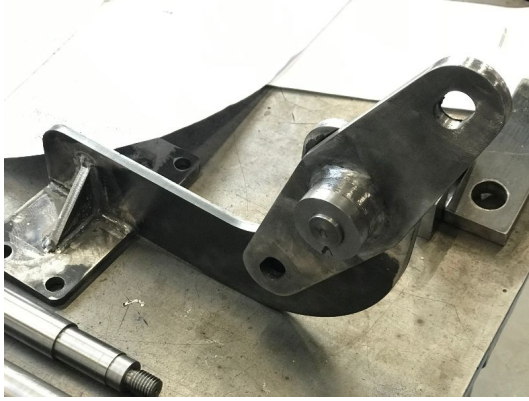
Cylinder drain cock linkage and rod ends- Bob Hughes/A1SLT
