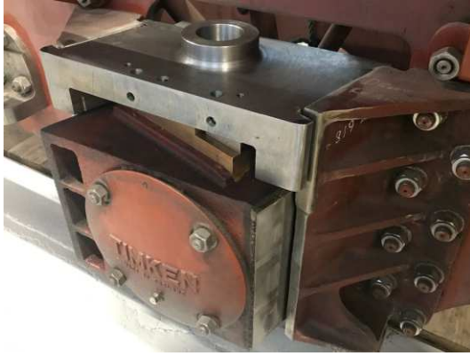
Cartazzi wheelset and spring plank assembly; pony truck frame fabrication - A1SLT
