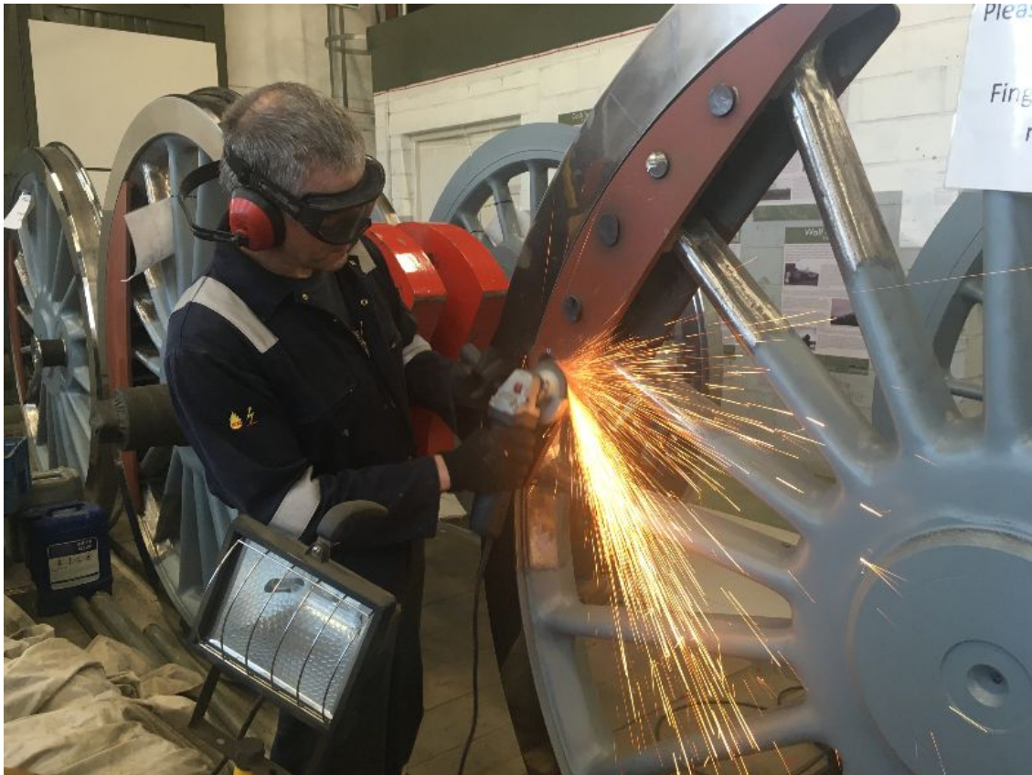
Ian Matthews grinding off the balance weight rivets on the intermediate wheelset- A1SLT
