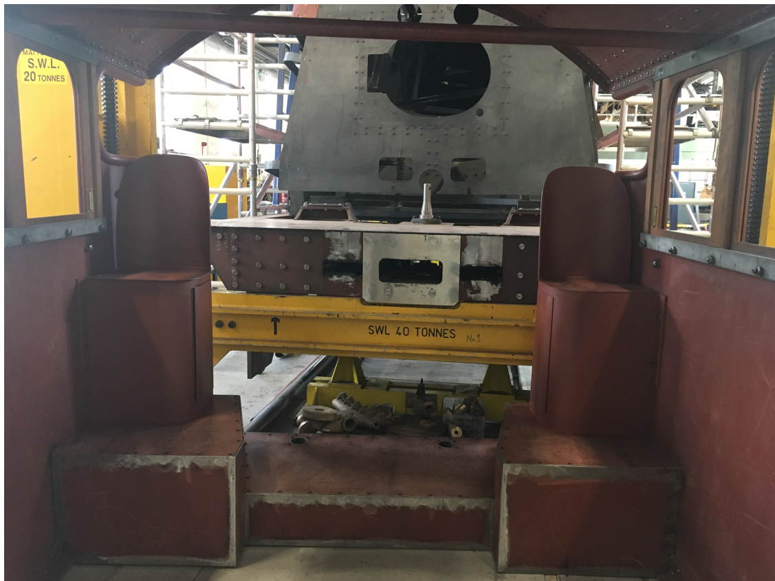
The driver's seat trial fitted in the cab, at DLW - A1SLT
