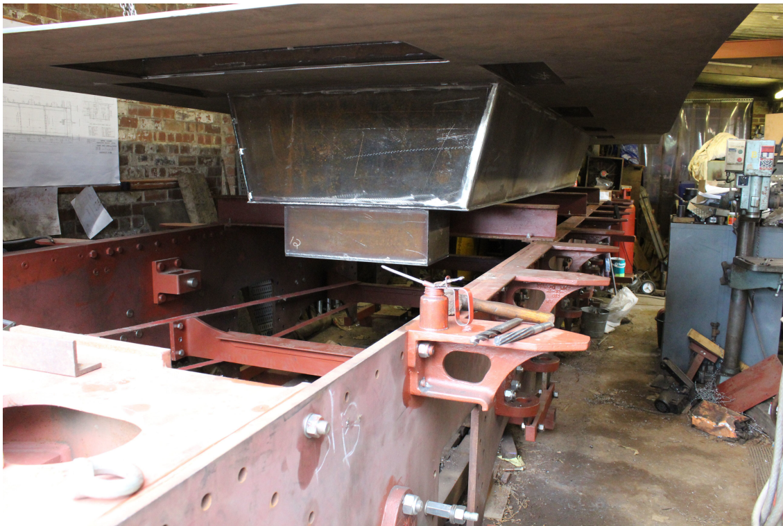
The tender baseplate being pre-fitted to the tender frames at I D Howitt, at Crofton- A1SL7
