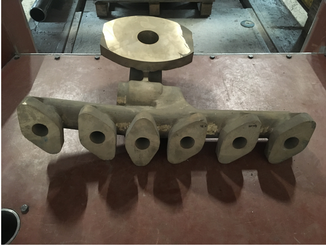
Steam stand casting, currently at DLW, ready for machining in the near future - A1SLT
