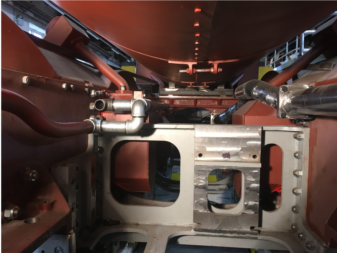
The vacuum pipe [left hand-side] and exhaust steam pipe [right-hand-side] inside the frames- A1SLT
