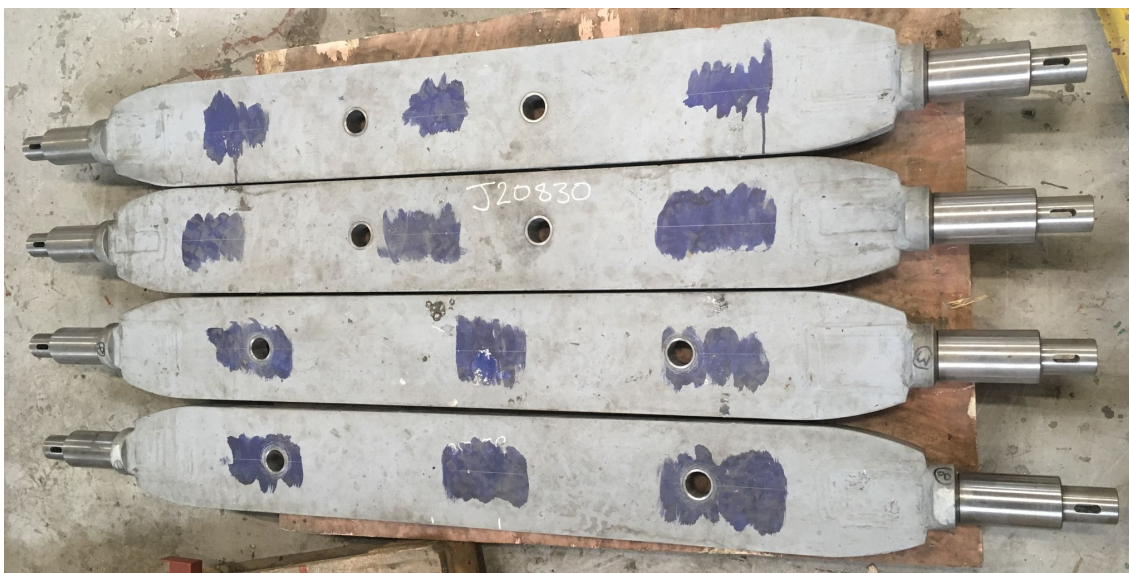
Brake stays which transmit the force from the brake cylinders to the brake hangers which carry the brake blocks - A1SLT
