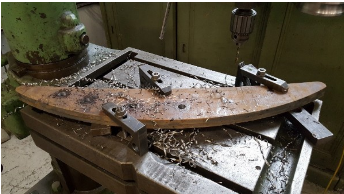
A pair of balance weights is machined at DLW - Ian Matthews
