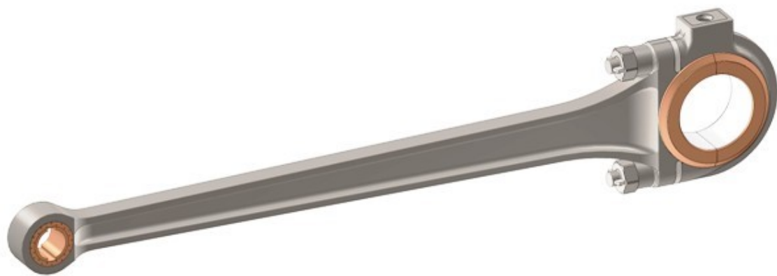
The inside connecting rod drawn in CAD - David Elliott
