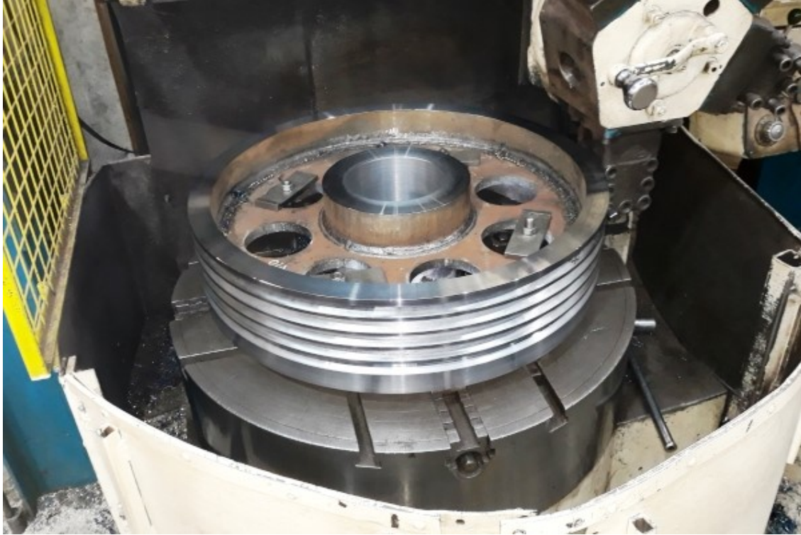
The tender alternator pulley being machined at North View Engineering - David Elliott
