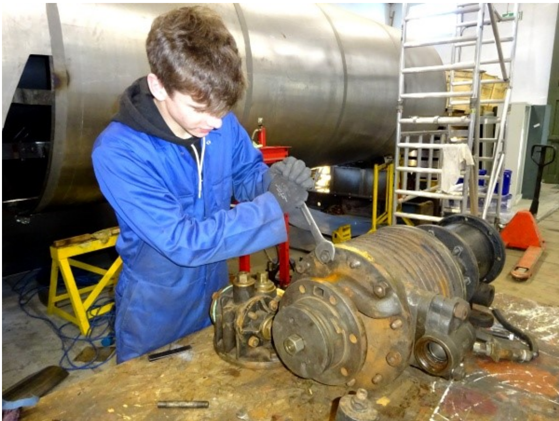
Jordan Durham from Middlesbrough College re-assembles an air pump - David Elliott
