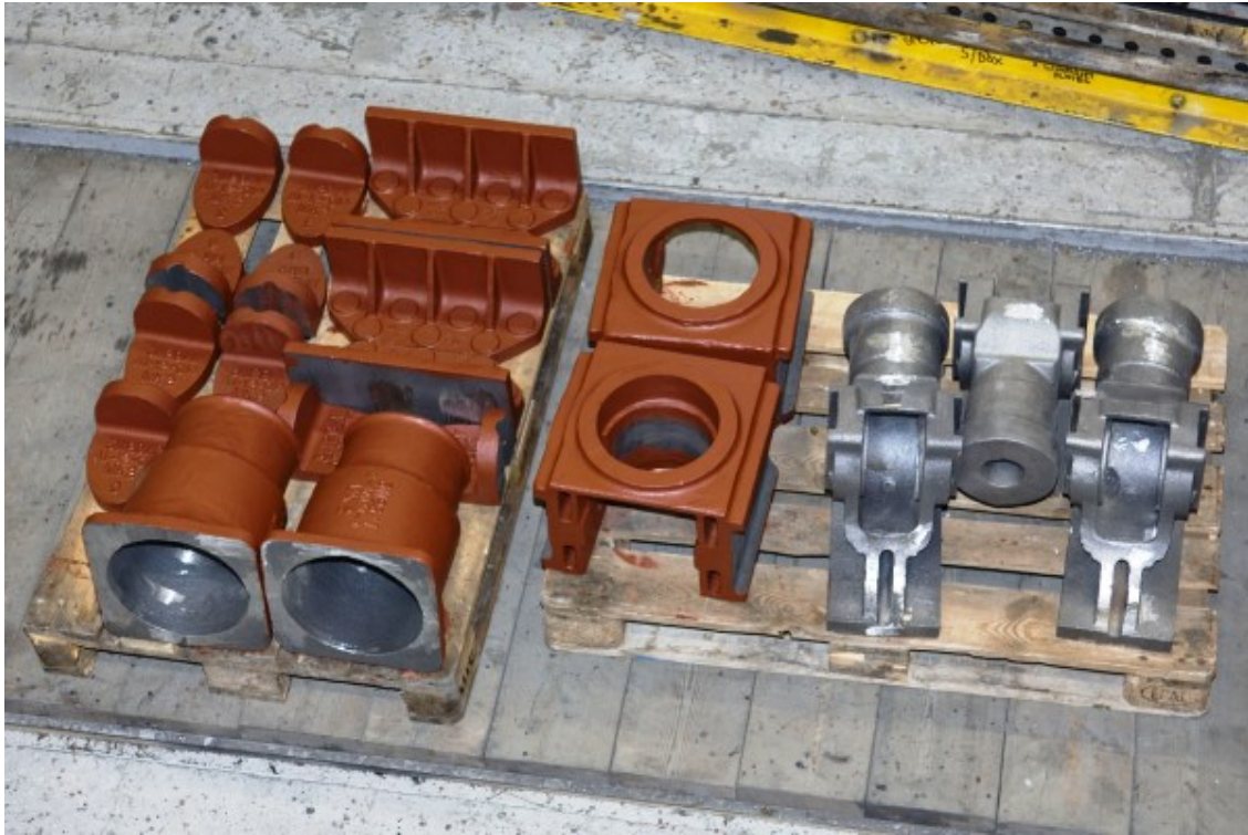
Tender castings ready for machining by Ian Howitt - Bob Hughes
