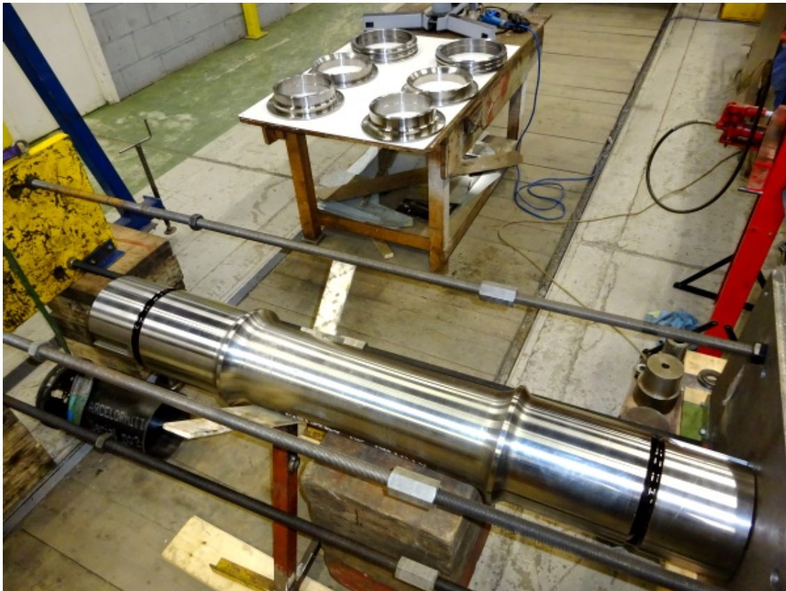
The leading axle set up on the bearing press - David Elliott
