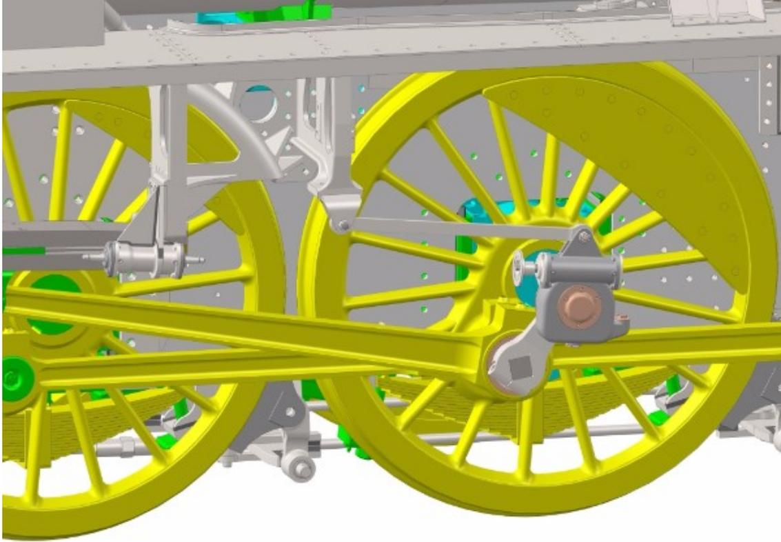
Elements of the valve gear are appearing on the CAD master drawing - *David Elliott*
