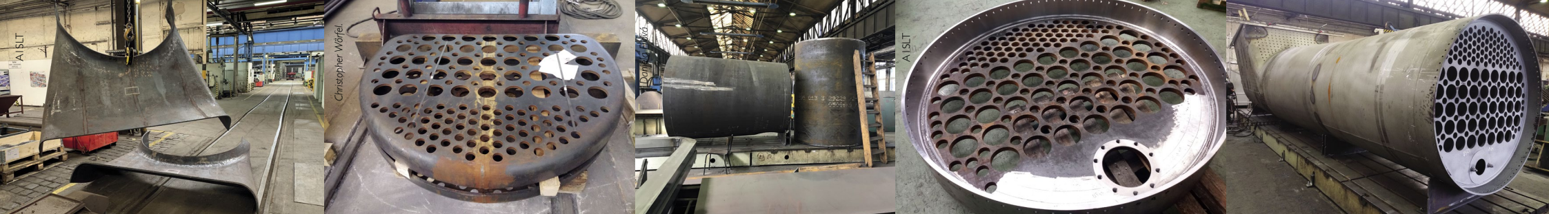
Inner and outer firebox throat plates at DBM. Firebox tube plates.
