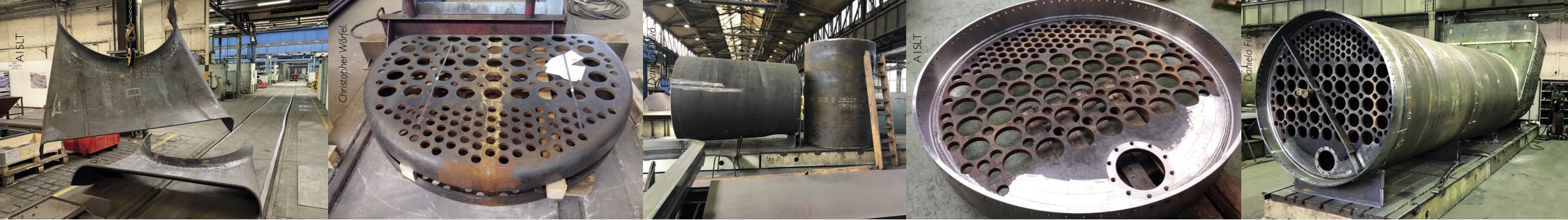
Inner and outer firebox throat plates at DBM. Firebox tube plates.
